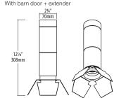
**FLX15-3040 :** FLEX fixture, 15W, 3000 K, 40° beam spread.
