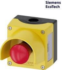
Enclosure for command devices, 22 mm, round, Enclosure material plastic, Enclosure top part yellow, 1 control point plastic, with protective collar, A=EMERGENCY STOP mushroom pushbutton red, 40 mm, rotate-to-unlatch, 1 NC, screw terminal, floor mounting, 1xM20 each on top and bottom
