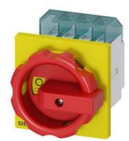
SENTRON, Switch disconnector 3LD, emergency switching-off switch, 3- pole, lu: 16 A, operating power / at AC-23 A 400 V: 7.5 kW, front-mounted, rotary operating mechanism, Red / yellow, 4-hole mounting of the handle
