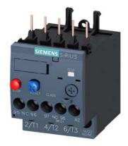
Overload relay 2.8...4.0 A Thermal For motor protection Size S00, Class 10 Contactor mounting Main circuit: Screw Auxiliary circuit: Screw Manual-Automatic-Reset
