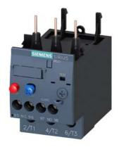
Overload relay 27...32 A Thermal For motor protection Size S0, Class 10 Contactor mounting Main circuit: Screw Auxiliary circuit: Screw Manual-Automatic-Reset
