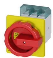
SENTRON, Switch disconnector 3LD, emergency switching-off switch, 3- pole, lu: 63 A, operating power / at AC-23 A 400 V: 22 kW, front-mounted, rotary operating mechanism, Red / yellow, central mounting 22.5 mm of the handle
