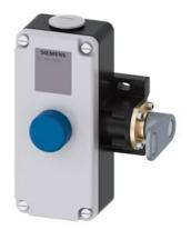
Cable-operated switch and lever Metal enclosure, 2 x M25 x 1.5; 2 NO+2 NC, latching EN ISO 13850 and pushbutton release, 2-sided operation for wire lengths up to 2 x 100 m  $^{\circ}$
