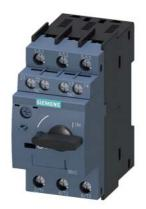
Circuit breaker size S00 for motor protection, CLASS 10 A-release 0.55...0.8 A N-release 10 A screw terminal Standard switching capacity with transverse auxiliary switches 1 NO+1 NC
