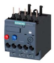
Overload relay 9.0...12.5 A Thermal For motor protection Size S00, Class 10 Contactor mounting Main circuit: Screw Auxiliary circuit: Screw Manual-Automatic-Reset
