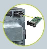
2 mini-slot ports for options using Network-M2 gives access to Eaton's software offerings
