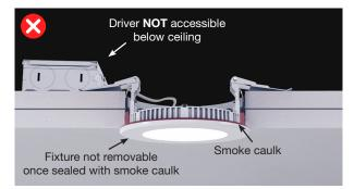
Fixture is smoke caulked, but no longer allows access to electrical connections below the ceiling.
