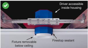
LUNA Fire maintains a fire barrier and allows for access to driver and electrical connections below the ceiling. Firestop sealant added between housing and ceiling only.
