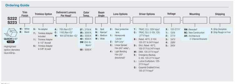
Delivered lumens provided are based on 3000 K with medium reflector. Not available with DTW. DTW models only. DTW models available in Non-IC only. Only available in 120V (Voltage option 1). 6 Not available in 347V. 7 Available with Delivered Lumens Per Head option; A or C only. 8 Ship complete only. 9 Only available with Driver Options "T" or "C"
