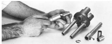
Figure 6. Wire Well Reducer Installation
