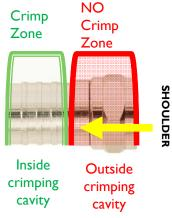
4) When crimping the connector, only crimp the areas below the shoulder ring.
