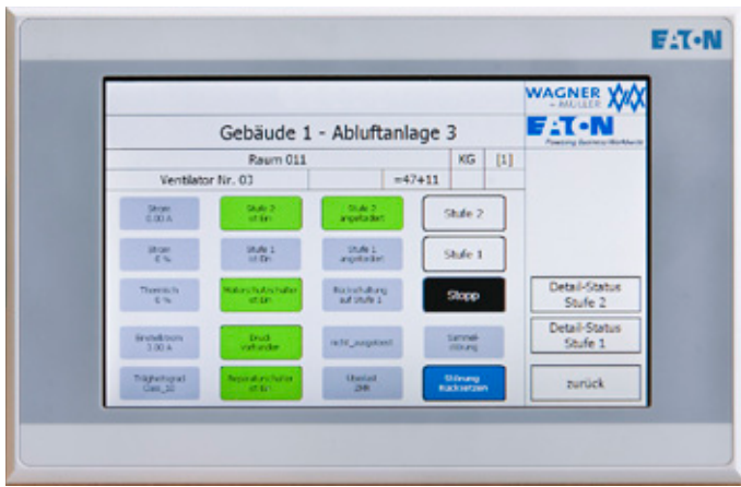
Clarity and convenience: both the operation and the control of the five systems are implemented with a 7.4 inch touch display PLC.
