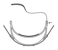
Once the elastic strap is adjusted comfortably, bend the ends of the face shield to slide the outer notches behind the back pegs of the head piece.
