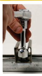
Installs 1/2" bolts into electrical strut channel for maximum strength. The Strutter Socket can be turned sideways, put into the strut, then slid over to the 1/2" bolt and tightened
