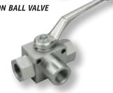
Note: Our Two-Position Ball Valves feature an L-pattern flow. Also known as a three-way valve or diverter valve, they can direct flow either to the left or to the right with a 90° turn of the handle.
