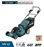
Cutting Width 480 mm (18-7/8") 20 - 100 mm (13/16 - 3-15/16") Cutting Height No Load Speed (RPM) 3,100 2.5 - 5.0 km/h w/BL1860B x2, Self-Propelled: 650 m<sup>2</sup> Propelling Speed Actual Mowing Area w/RI 1860R x2 Push-Drive: 800 m<sup>2</sup> w/BL1860B x2, Continuous Use (min.) Self-Propelled: 23 w/BL1860B x2, Push-Drive: 28 During Operation: 1,690 - 1,740 x 530 x 930 - 1,060 mm Dimensions (LxWxH)Net weiaht 27.1 - 29.3 ka
