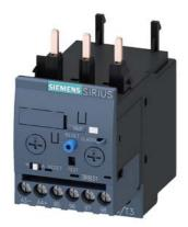
Overload relay 3...12 A Electronic For motor protection Size S0, Class 5...30 Contactor mounting Main circuit: Screw Auxiliary circuit: Screw Manual-Automatic-Reset Internal ground fault detection
