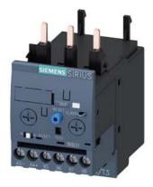
Overload relay 0.32...1.25 A Electronic For motor protection Size S0, Class 5...30 Contactor mounting Main circuit: Screw Auxiliary circuit: Screw Manual-Automatic-Reset Internal ground fault detection
