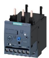
Overload relay 10...40 A Electronic For motor protection Size S0, Class 10E Contactor mounting Main circuit: Screw Auxiliary circuit: Screw Manual-Automatic-Reset
