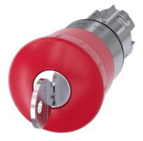
EMERGENCY STOP mushroom pushbutton, 22 mm, round, metal, shiny, red, 40 mm, with RONIS lock, lock number SB30, positive latching, acc. to EN ISO 13850, key-operated release
