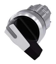
Selector switch, illuminable, 22 mm, round, metal, shiny, white, selector switch, long, 2 switch positions O<I, momentary contact type, Actuating angle 45°, 10:30h/12h
