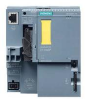
SIMATIC DP, CPU 1512SP F-1 PN for ET 200SP, Central processing unit with Work memory 300 KB for program and 1 MB for data, 1st interface: PROFINET IRT with 3-port switch, 48 ns bit performance, SIMATIC Memory Card required, BusAdapter required for Port 1 and 2
