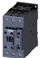
power contactor, AC-3e/AC-3, 51 A, 22 kW / 400 V, 3-pole, 110 V AC, 50 Hz / 120 V, 60 Hz, auxiliary contacts: 1 NO + 1 NC, screw terminal, size: S2  $\,$
