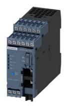
basic unit SIMOCODE pro V PN, Ethernet/PROFINET IO, PN system redundancy, OPC UA server, web server, transfer rate 100 Mbps, 2 x bus connection via RJ45, 4I/3O freely parameterizable, US: 110 - 240 V AC/DC, input for thermistor connection monostable relay outputs, expandable by expansion modules
