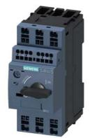
Circuit breaker size S00 for motor protection, CLASS 10 A-release 2.2...3.2 A N release 42 A Spring-type terminal Standard switching capacity with transverse auxiliary switches 1 NO+1 NC  $\,$
