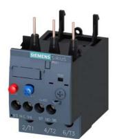
Overload relay 23...28 A Thermal For motor protection Size S0, Class 10 Contactor mounting Main circuit: Screw Auxiliary circuit: Screw Manual-Automatic-Reset
