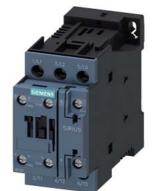
power contactor, AC-3e/AC-3, 32 A, 15 kW / 400 V, 3-pole, 24 V DC, auxiliary contacts: 1 NO + 1 NC, screw terminal, size: S0
