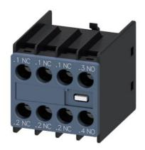
auxiliary switch, on the front, 1 NO + 3 NC, .1/.2, .1/.2, .1/.2, .3/.4, current path: 1 NC, 1 NC, 1 NO, screw terminal, for contactors 3RT2 and contactor relays 3RH2
