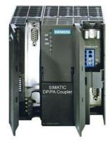
SIMATIC DP, distributed I/O Field device interface DP/PA coupler Ex version Ex(IA) 110 mA Field coupler between PROFIBUS DP and field bus segments to IEC 61158-2, for example PROFIBUS PA, for extended temperature range Degree of protection IP20
