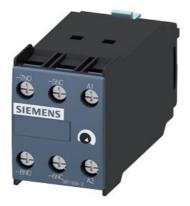
solid-state time-delayed front-side auxiliary switch Time range 0.5...10 s, 200 ... 240 V AC / DC, 1 NO contact, 1 NC contact OFF delay, without control signal for 3RT1
