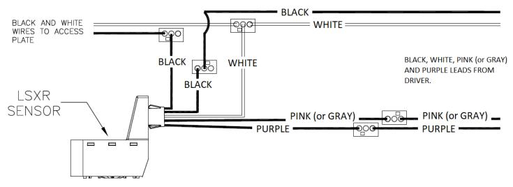
Figure 3: LSXR10 Wiring Diagram
