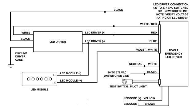
Figure 1: PS1055LCP Wiring Diagram
