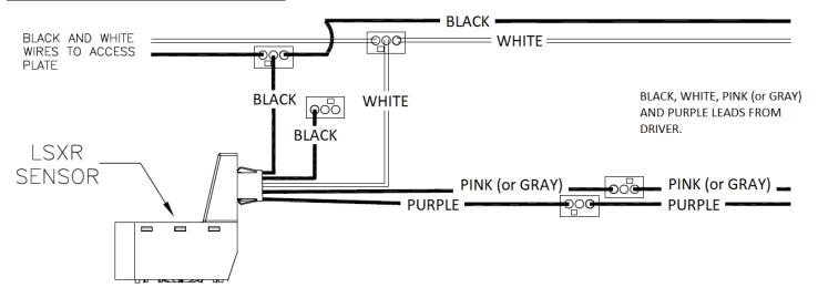
Figure 4: LSXRHL Wiring Diagram
