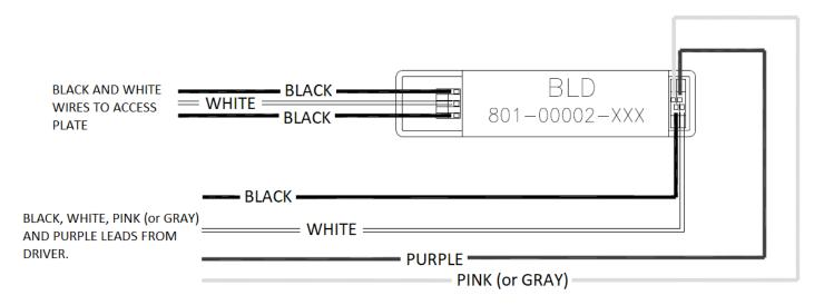
Figure 5: SLD Wiring Diagram
