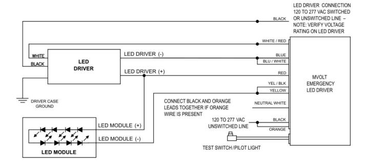
Figure 2: EL7L/14L Wiring Diagram
