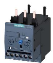
Overload relay 6...25 A Electronic For motor protection Size S0, Class 5...30 Contactor mounting Main circuit: Screw Auxiliary circuit: Screw Manual-Automatic-Reset Internal ground fault detection
