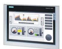
SIMATIC HMI TP1200 Comfort, Comfort Panel, touch operation, 12" widescreen TFT display, 16 million colors, PROFINET interface, MPI/PROFIBUS DP interface, 12 MB configuration memory, Windows CE 6.0, configurable from WinCC Comfort V11
