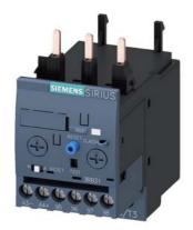
Overload relay 1...4 A Electronic For motor protection Size S0, Class 5...30 Contactor mounting Main circuit: Screw Auxiliary circuit: Screw Manual-Automatic-Reset Internal ground fault detection
