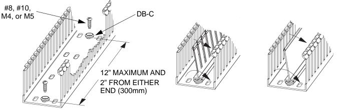
REMOVING FINGERS ON SLOTTED DIVIDER WALL
