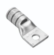
Copper Compression Lug, Ring Tongue, 1 Hole w/ Inspection Window, AN 5 & 6 Flex, 5/16" Stud, Short Barrel, Tin Plated.
