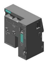
SIMATIC DP, IM151-8 PN/DP CPU f. ET200S, 192 KB work memory, int. PROFINET interface (with three RJ45 ports) as IO controller, without battery MMC required
