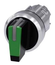
Selector switch, illuminable, 22 mm, round, metal, shiny, green, selector switch, short, 3 switch positions I-O-II, latching, actuating angle  $2x45^\circ$ , 10:30h/12h/13:30h
