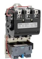
Non-reversing motor starter Size 3 1/2 Three phase full voltage Solid-state overload relay OLRelay amp range 50-200A 110VAC 50HZ / 120VAC 60HZ coil Combination type No enclosure
