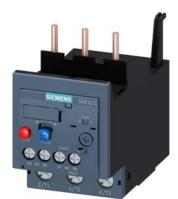
Overload relay 18...25 A Thermal For motor protection Size S2, Class 10 Contactor mounting Main circuit: Screw Auxiliary circuit: Screw Manual-Automatic-Reset
