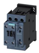
power contactor, AC-3e/AC-3, 25 A, 11 kW / 400 V, 3-pole, 110 V AC, 50 Hz / 120 V, 60 Hz, auxiliary contacts: 1 NO + 1 NC, screw terminal, size: S0
