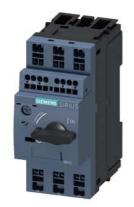
Circuit breaker size S00 for motor protection, CLASS 10 A-release 2.8...4 A N release 52 A Spring-type terminal Standard switching capacity with transverse auxiliary switches 1 NO+1 NC
