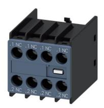
auxiliary switch, on the front, 4 NC, .1/.2, .1/.2, .1/.2, .1/.2, current path: 1 NC, 1 NC, 1 NC, 1 NC, screw terminal, for contactors 3RT2 and contactor relays 3RH2
