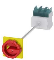
SENTRON, Switch disconnector 3LD, emergency switching-off switch, 3- pole, lu: 125 A, operating power / at AC-23 A 400 V: 45 kW, floor mounting with door coupling, rotary operating mechanism, Red / yellow, 4-hole mounting of the handle
