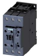
power contactor, AC-3e/AC-3, 80 A, 37 kW / 400 V, 3-pole, 24 V AC, 50/60 Hz, auxiliary contacts: 1 NO + 1 NC, screw terminal, size: S2  $\,$
