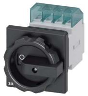
SENTRON, Switch disconnector 3LD, main switch, 3-pole, lu: 16 A, Operating power / at AC-23 A at 400 V: 7.5 kW, front-mounted, rotary operating mechanism, black, central mounting 22.5 mm of the handle
