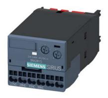
solid-state time-delayed auxiliary switch, off delayed, without control signal, relay 1 NC + 1 NO, time range 0.05-100 s, 24-240 V AC/DC, 50/60 Hz, varistor for attenuation of the contactor coils integrated, spring-loaded terminal, can be snapped on at the front on contactors 3RT2 and auxiliary contactors 3RH2
